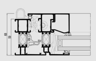
Concept System® 68 is a thermally improved three-chamber system for windows and doors that boasts the optimum combination of high insulation levels and optimal safety.
